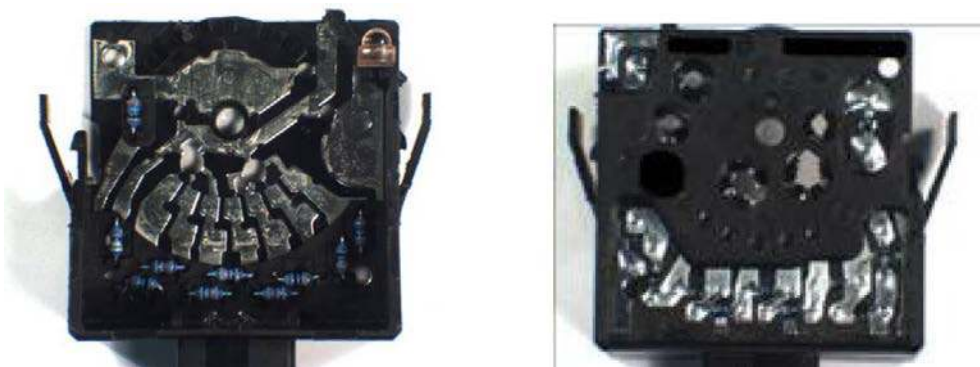
Fig. 6: Lead frame for a control knob to adjust the headlight height left: topside right: downside
