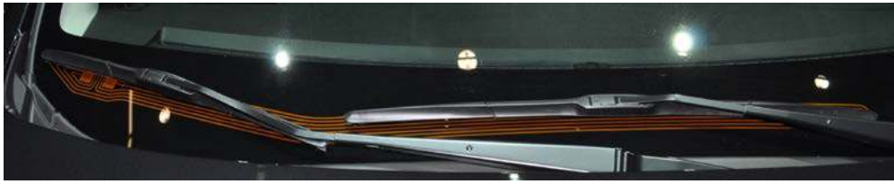
Fig. 39: windscreen wiper heating on laminated glass
