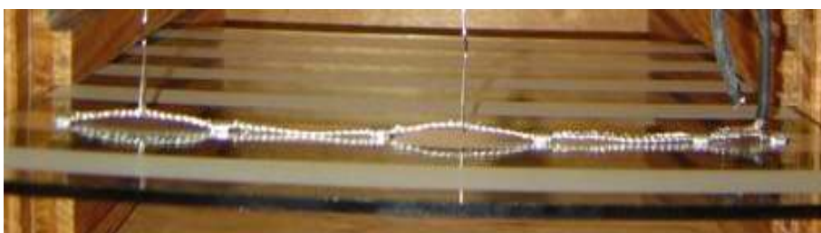
Fig. 32: Soldered braids are another type of connectors
