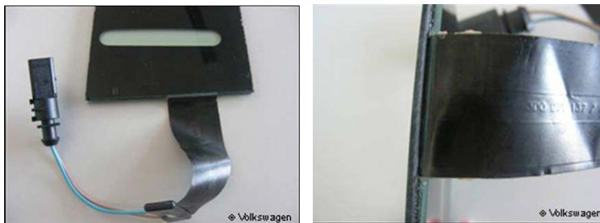
Fig. 37: Example for a lead solder application at laminated glazing structure
